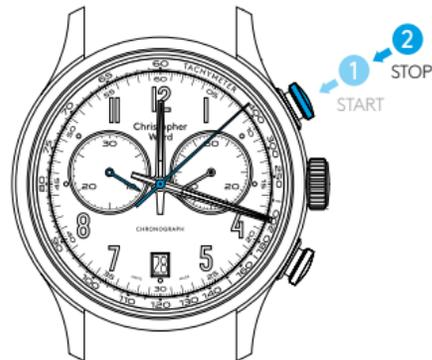
To stop the timing, press push-button **A** once more and read the 2 chronograph counters, for example: 10 mins / 8 seconds.
