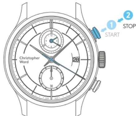
To stop the timing, press **push-button A** once more and read the three chronograph hands, for example: 2 hours/10 mins/20 seconds.
