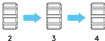
For a superior water resistance your crown is of the screw-in type. The crown should sit flush to the case (position **1**) in order to maintain water resistance.
