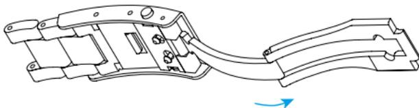
3. There are five micro adjustment positions, which allows for a maximum extension of 8.4mm. To extend, pull the lever to unlock and simultaneously pull on the bracelet into the desired position.
