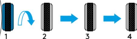
For a superior water resistance your crown is of the screw-down type. The crown should sit flush to the case (position **1**) in order to maintain water resistance.
