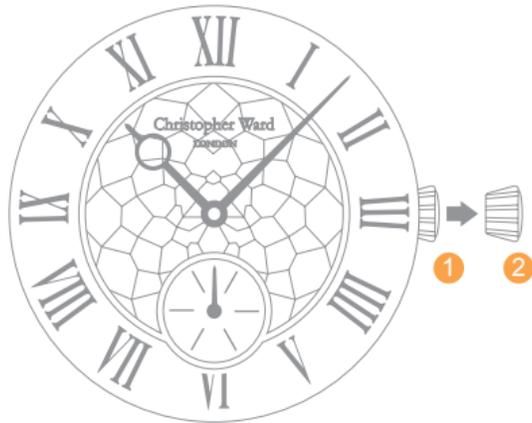
Pulling the crown out to position ②, stops the secondhand
