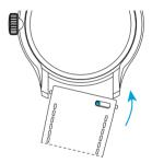
**2.** To reattach your strap, align the pins to the lug holes and click the strap into position. Repeat for the other side.
