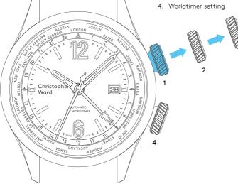
The crown should sit flush to the case (position **1**) in order to maintain water resistance.
