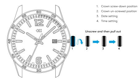
For a superior water resistance your crown is of the screw-down type. The crown should sit flush to the case (position 1) in order to maintain water resistance.
