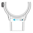
**1.** Locate the quick-release pin on your strap. Pull the pin to the side to detach your strap.
