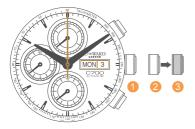
• Pull out the crown to position (3) (the watch stops).
