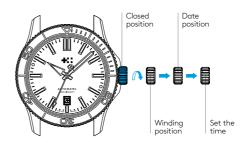
Date correction should not be carried out between 20.00 hr and 02.00 hr as the watch gearing will already be aligning itself to change the date.
