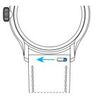
**1.** Locate the quick-release pin on your strap. Pull the pin to the side to detach your strap.
