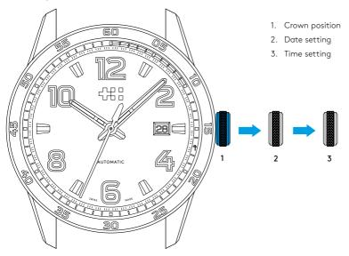
The crown should sit flush to the case (position 1) in order to maintain water resistance.
