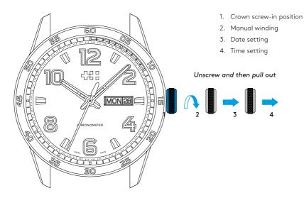
For a superior water resistance your crown is of the screw-in type. The crown should sit flush to the case (position 1) in order to maintain water resistance.
