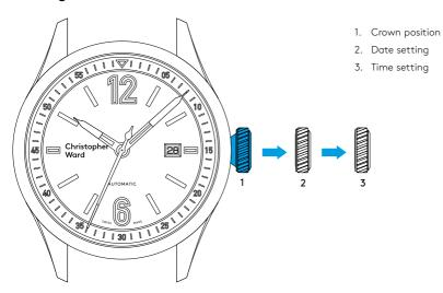
The crown should sit flush to the case (position 1) in order to maintain water resistance.
