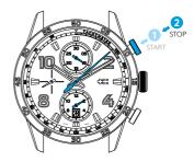
To stop the timing, press push-**button A** once more and read the 3 chronograph counters, for example: 2 hours/10 mins/8 seconds.
