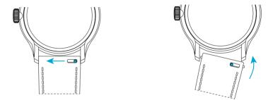
Locate the quick-release pin on your strap. Pull the pin to the side to detach your strap. **2.** To reattach your strap, align the pins to the lug holes and click the strap into position. Repeat for the other side.
