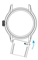
To reattach your strap, align the pins to the lug holes and click the strap into position. Repeat for the other side.
