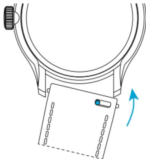
2. To reattach your strap, align the pins to the lug holes and click the strap into position. Repeat for the other side.
