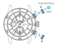
First unscrew the pushers anti-clockwise from the case into position **2** for starting, stopping, restarting and resetting the timing mode.
