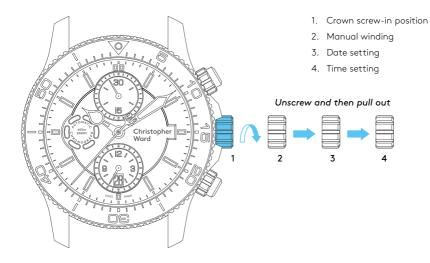
For a superior water resistance your crown is of the screw-in type. The crown should sit flush to the case (position 1) in order to maintain water resistance.
