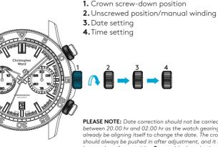
PLEASE NOTE: Date correction should not be carried out between 20.00 hr and 02.00 hr as the watch gearing will already be aligning itself to change the date. The crown should always be pushed in after adjustment, and it is best to do so from position **3** to avoid advancing beyond the desired date
