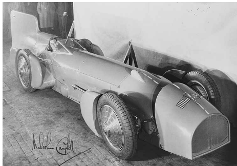
Above; Malcolm Campbell in his supercharged 26.9-litre Napier powered Bluebird which reached 246mph in 1931.
