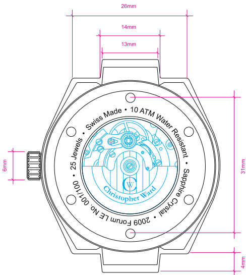
316L Stainless Steel brushed finish Sapphire Crystal - underside anti-reflective coating
