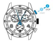
To stop the timing, press push-**button A** once more and read the 12 hour counter, 60 minutes counter, 60 seconds counter and 1/10 second counter. For example: 5 mins, 57 seconds and 7/10 second.
