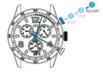
To restart the timing, press push-**button A** again (timing is resumed).
