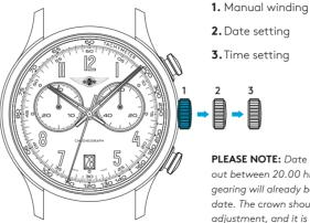
**3.** Time setting **PLEASE NOTE:** Date correction should not be carried out between 20.00 hr and 02.00 hr as the watch gearing will already be aligning itself to change the date. The crown should always be pushed in after adjustment, and it is best to do so from position 3 to avoid advancing beyond the desired date.
