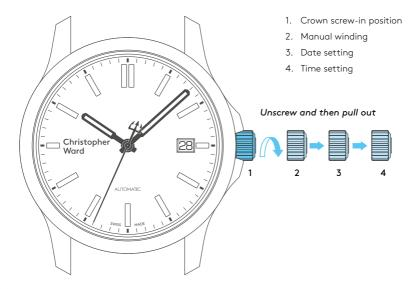
For a superior water resistance your crown is of the screw-in type. The crown should sit flush to the case (position 1) in order to maintain water resistance.
